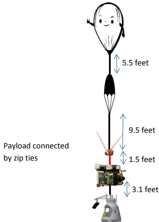
**Figure 8:** Payload Train Schematic
