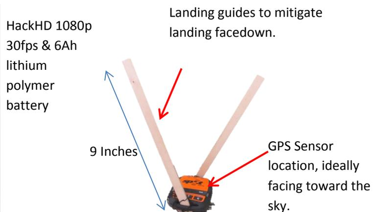
**Figure 7:** SPOT GPS with Landing Guides
