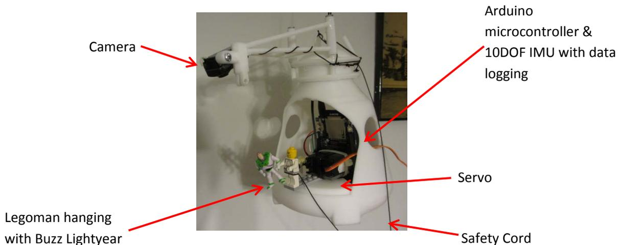
**Figure 3:** 3D Printed Capsule with boom (10% infill, 0.31mm layer height)
