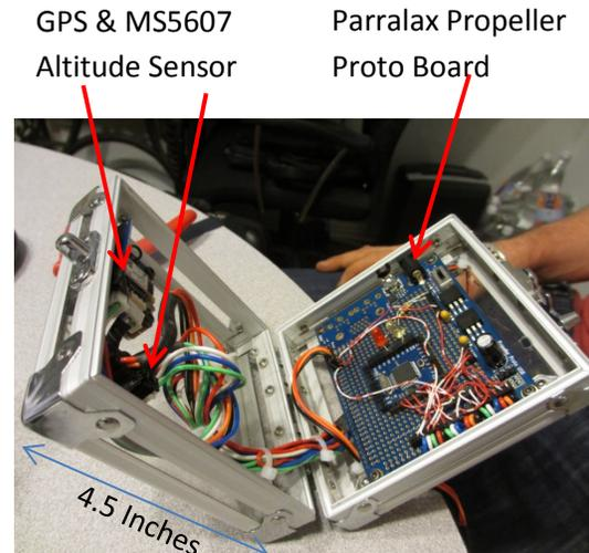
**Figure 5:** Internal Electronics and sensors
